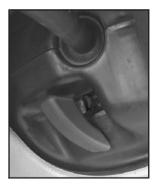
To tilt the wheel, hold the steering wheel and pull the lever. Move the steering wheel to a comfortable level, then release the lever to lock the wheel in place.
